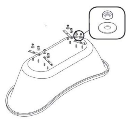
3. Take a short bar and place it over the bolts on the bottom of the tub & use the 11/16" washer, lock washer, and nut (In that order) on the bolt coming through the bar on the tub.
