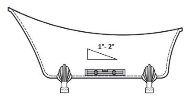
20. Place a level inside the tub. Make sure the bathtub is stable and that all legs rest perfectly on the floor, if not, ad-just the levelling pads.
